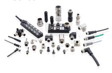
Amphenol LTW M Series Sensor Connectors feature waterproof ratings of IP65, IP67, IP68 and IP69K with current ratings of 1.5A to 28A. This connector series includes receptacles, connectors overmolded with cable, and field-installable connectors with at least 100 mating cycles. Amphenol LTW M Series connectors meet IEC standards. These connectors offer standard cable lengths ranging from 1M to 99M. These sensor connectors are also available in M8 SMT and M12 SMT models.
