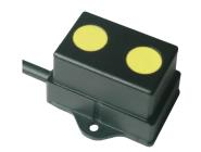
The Telaire T3000 Series CO<sub>2</sub> sensors are designed for CO<sub>2</sub> monitoring in harsh and demanding environments. Utilizing Telaire's nondispersive infrared (NDIR) sensor and electronic signal conditioning technology, the T3000 Series provides robust packaging in numerous configurations of measurement range, supply voltage, and output signals.
